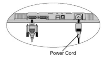
To input the Signal through ADC
